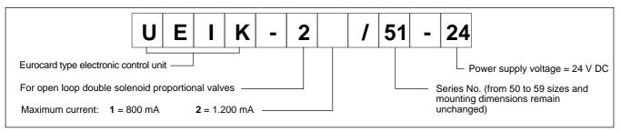
The UEIK-2\* card is an electronic control unit Eurocard type for open loop of double solenoid proportional valves.
